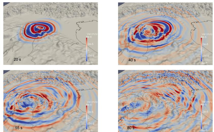
Snapshots at 20 s, 40 s, 55s (left) and 80s (right) after the 27 Jan. 2012 earthquake ( $M_w=5.4$ ). Half duration was set to 1.8 s.
