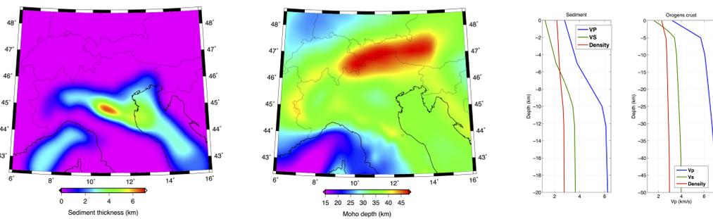
(left) Sediment layer thickness (km) arranged from literatures, (right) Moho depth taken from EPcrust (Molinari & Morelli, 2011)
