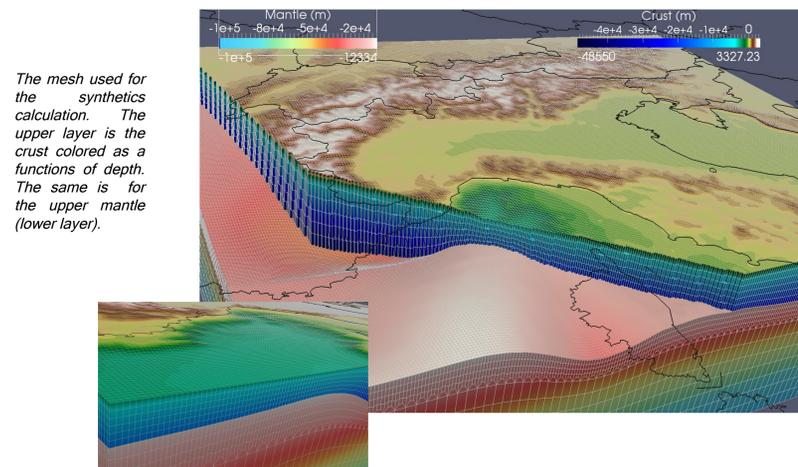
The mesh used for the synthetic calculation. The upper layer is the crust colored as a function of depth. The same is for the upper mantle (lower layer).
