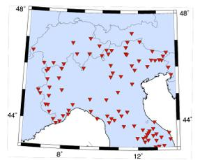
Seismic station distribution in the Po Plain area, available for a noise tomographic study.
