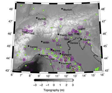
Historical seismicity between 1000 AD to 1970 AD with intensity larger than 5.5. Green dots represent the instrumental earthquakes recorded from 1970 to 2012 with magnitude bigger than 4.
