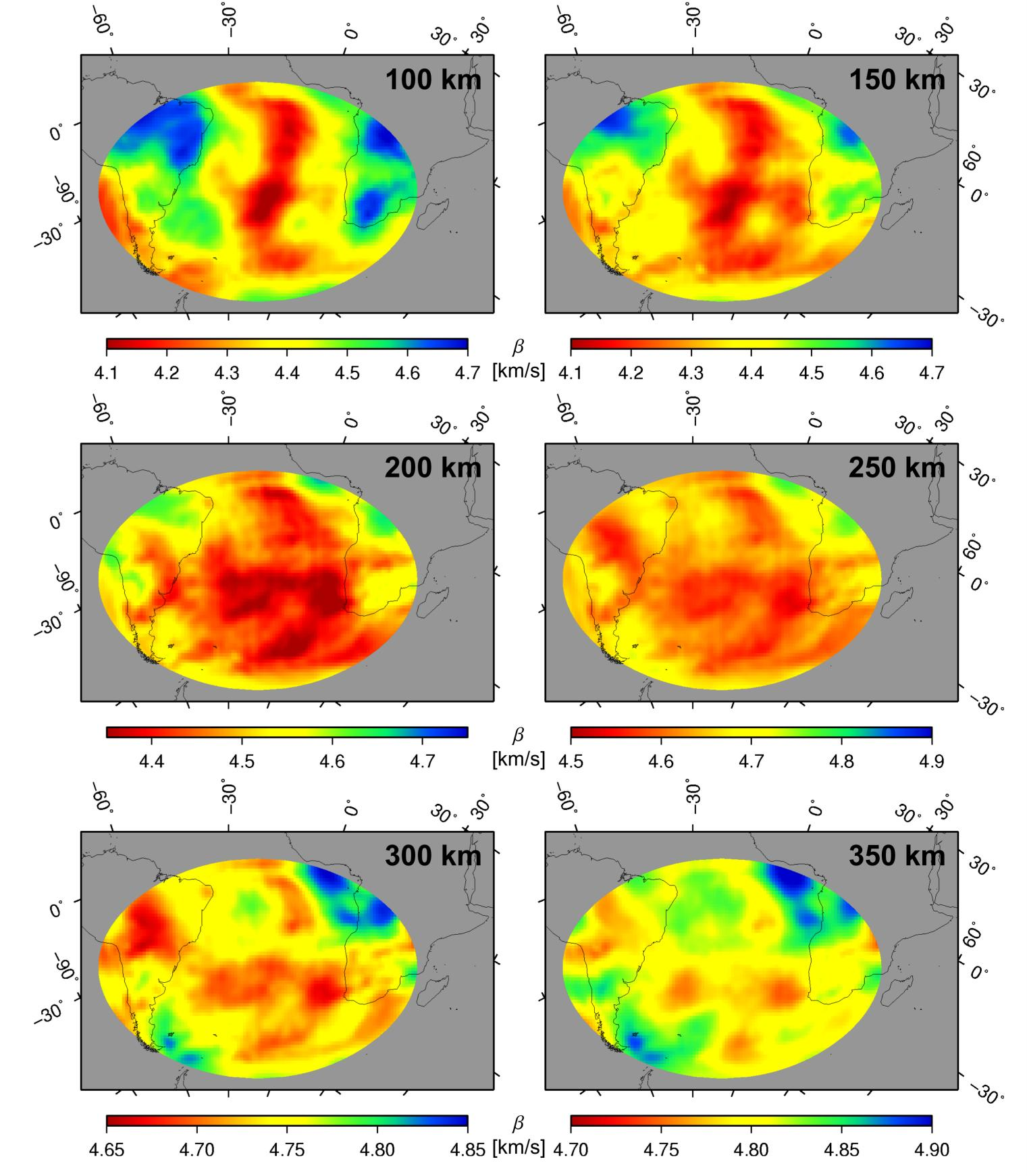
Horizontal slices of the S velocity model at six different depths. At 150 km depth the velocity anomalies are still strongly influenced by the chemical composition and thermodynamic evolution of the lithosphere. Between 200 and 300 km depth the mantle is dominated by slow, elongated anomalies, while deeper than 300 km the slow anomalies become more rounded, possibly related to columnar upwelling material coming from deeper in the mantle.
