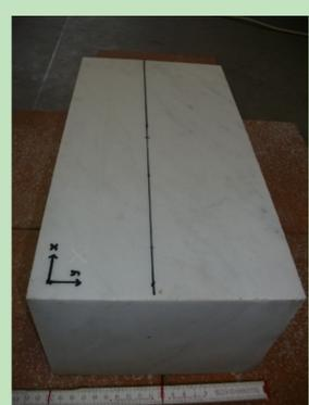
**Figure 6:** 400X205X150 mm marble sample investigated with an ultrasonic non-destructive technique.
