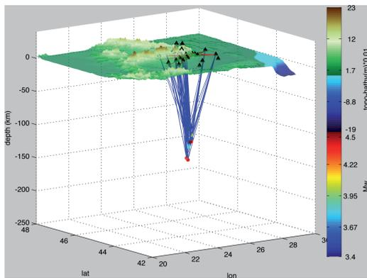
Our database is built on the broad-band data records from the 1999 CALIXTO experiment which took place in Vrancea for 6 months. It consists of 21 events with magnitude from Mw=3.2 to Mw=4.5, at depth ranging from 15km to 154km recorded at least by 3 stations.
