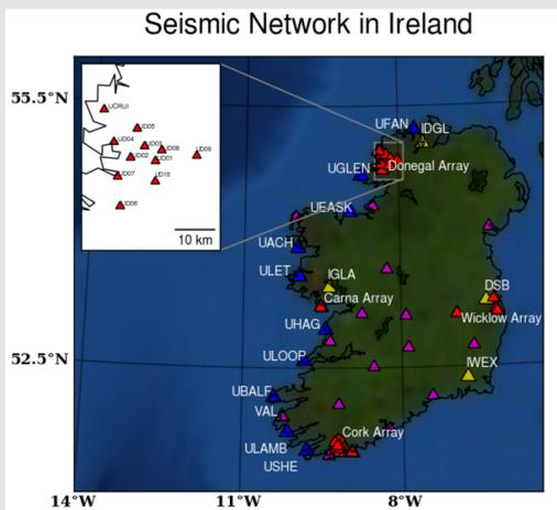
Figure 1: Seismic network deployed in Ireland; the blue and red stations are operated by UCD. The pink stations are deployed by the Dublin Institute for Advanced Studies (DIAS).
