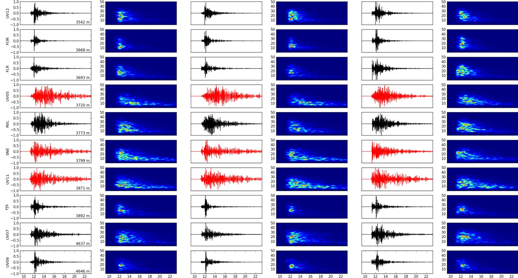
The waveforms of the stations on the summit emulate VT-B events; no distinction between P- and S-wave onset, emergent wave-trains with the main part of the energy shifted to later times, reduction of the maximum amplitude and a considerable lack of the high frequency content.
