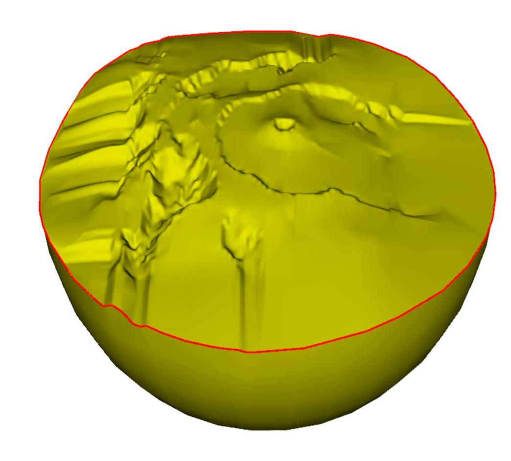
Starting from a DEM the **geometry** is created bottomup: refers to an approach where one first creates the vertices, connects those to form edges and connects the edges to create faces. In order to avoid boundary reflections we enlarge the geometry applying a Gaussian taper. The intersection of this surface with a sphere finally creates the geometry.
