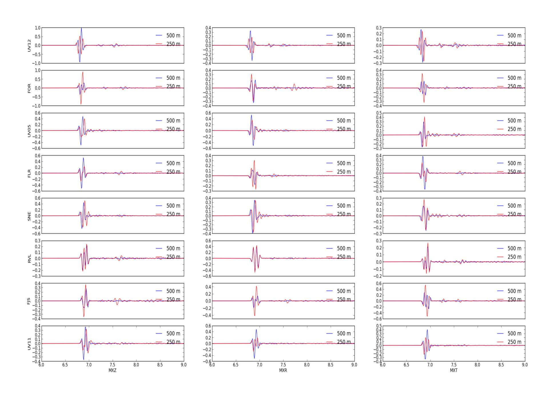
We compare two simulations with different topography resolutions (500 m and 250 m), using an event 1190 m bsl and located just below the summit (the same one that section Scattering at Piton de la Fournaise shows). We use an explosive source mechanism. The highest frequency our numerical domain can resolve is 10 Hz.
